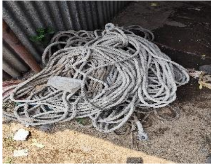
Damaged lifeline rope
