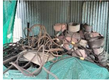
Old and damaged web slings
