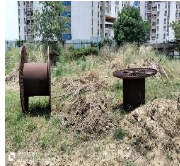
MS electrical cable drum (empty)
