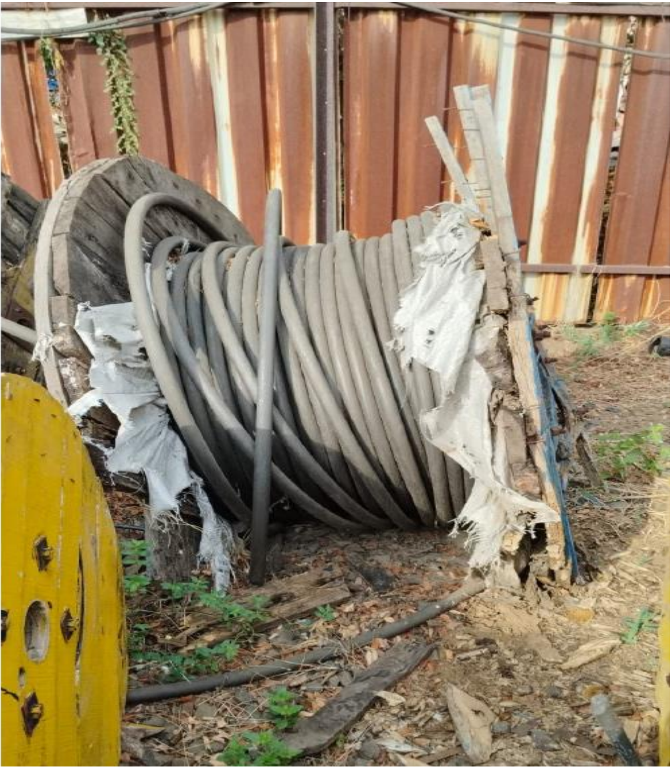
ALUMINIUM CABLE SIZE 1CX 95 SQMM
