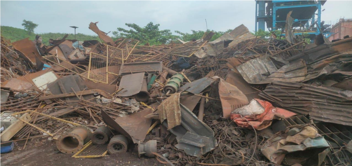
Light melting mixed with jumbled TMT, crushed corrugated & Collecting sheet , filter cages etc
