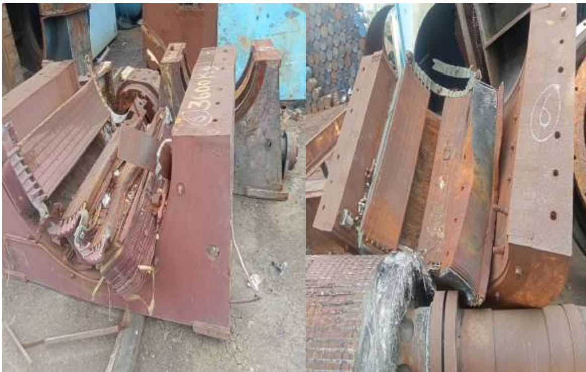
S. NO. 13 EXCITER STATOR - CARBON STEEL+COPPER (10%)– 5.8 MT
