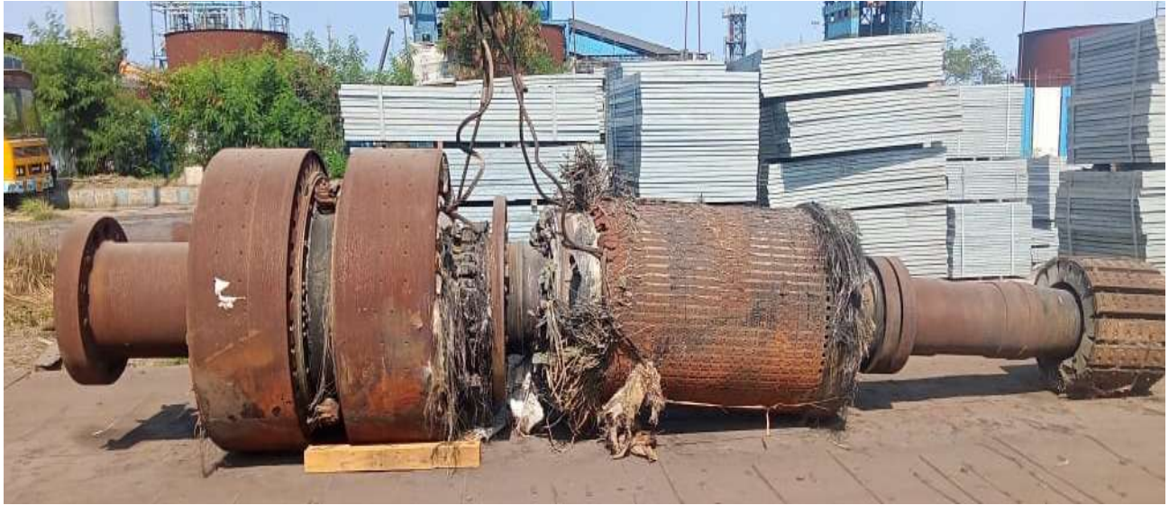
S. NO.10 EXCITOR ROTOR ALLOY STEEL – P11 + INSIDE COPPER (10%)- 7.29 MT
