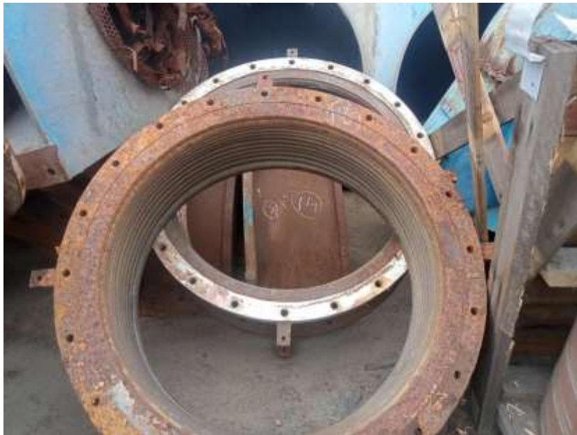
S.NO. 23 TURBINE BELLOW – CARBON STEEL+ SS – 0.45MT
