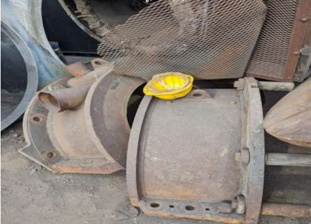
S.NO. 22 TURBINE DIAPHARAGM - CARBON STEEL – 2.95 MT
