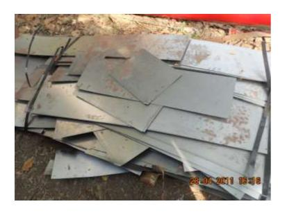
CR MIXED CUT SHEETS (GENERATED FROM MBL & CTL, AFTER SLITING CRS FOLDED SHEET & 10% HRPSO SHEET) THIS MATERIAL MAY HAVE DEFECTS ON SURFACE/EDGES 1% MATERIAL 50 MM WITH INCLUDING IN TOTAL QTY.INCLUDING MINOR RUST. M.NO. 35601(STOCK + ARISING)
