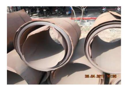
CR BABY STICK COILS-(UNSKINPASS COILS, HIGH HARDNESS, STICKY WRAPS) M. NO. 294867 (STOCK + ARISING)
